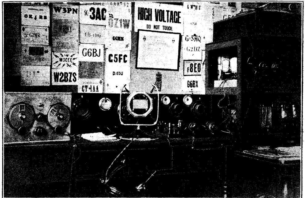
A QUALITY TRANSMITTER. G2QH, owned and operated by Mr. C. Hewins, Grimsby, Lincs. On the extreme right is the speech amplifier and 100 per cent. modulator and power equipment. Behind the Reisz "mike" is the crystal-controlled transmitter. The short-wave receiver is on the left.
